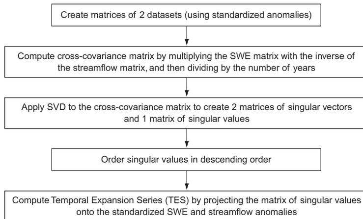
Figure 4. Flowchart illustrating the steps involved in SVD.
