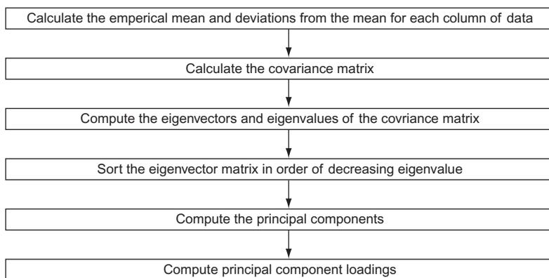
Figure 2. Flowchart illustrating the steps involved in PCA.
