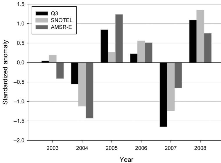
Figure 3. April–May–June–July streamflow versus 1 April snowpack (2003–2008). Standardized SWE from a single SNOTEL station and its corresponding AMSR-E grid cell are plotted against standardized streamflow (Q3).
